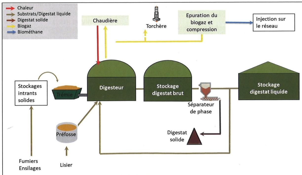
SCHEMA DE PRINCIPE DE L'INSTALLATION DE METHANISATION
